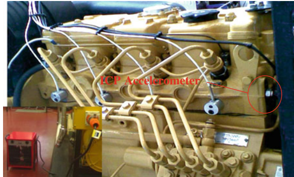
Fig. 34.1 A graphical illustration of the four-stroke, four-cylinder diesel engine test rig and the attached sensors
